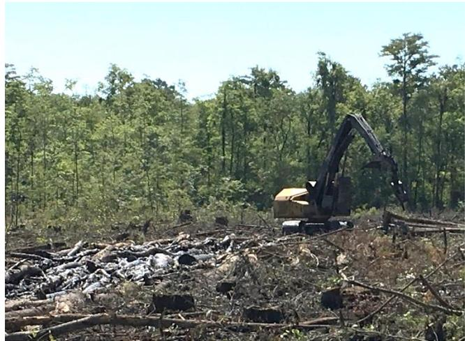
*Right: A track-mounted log-loader (called a shovel logger, or shovel machine), on the end of a shovel skid trail.*
